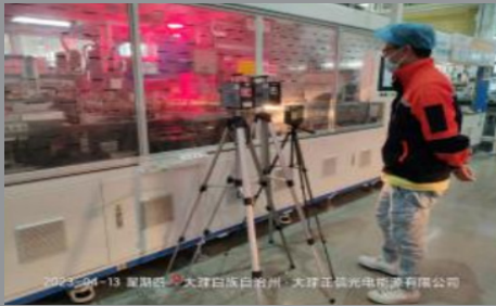
Chemical Detection of String Welder Fixed Spots
